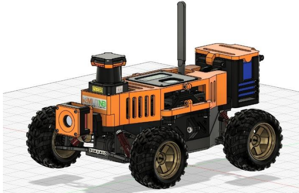
Fig. 4. Ground-based wheeled drone used to record energy consumption during route execution.
