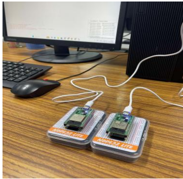
Fig 7. Prototype system setup for firmware testing and validation, showing two ESP32 development boards connected via USB to a host computer.
