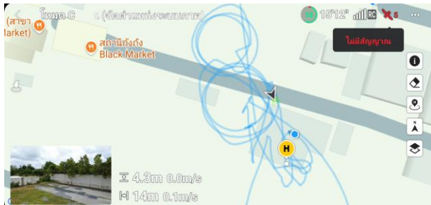
Fig. 15 . Drone lost GPS signal
